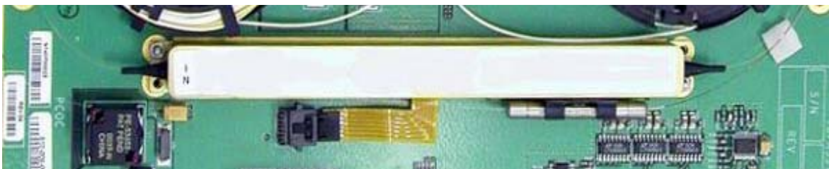
Figure 2. Adaptive dispersion compensator is a compact device sitting on the receiver board in each 40Gb/s transponder.
